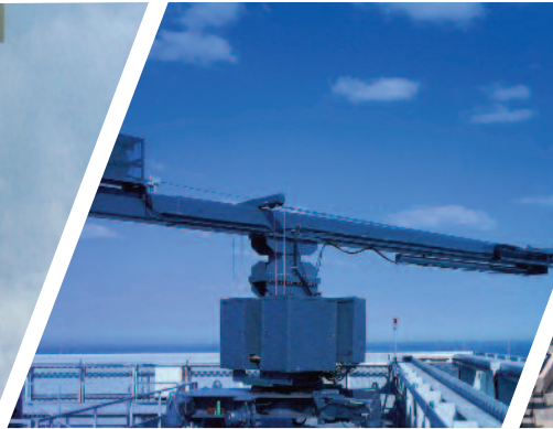
Material Hoist at Boom Tip
